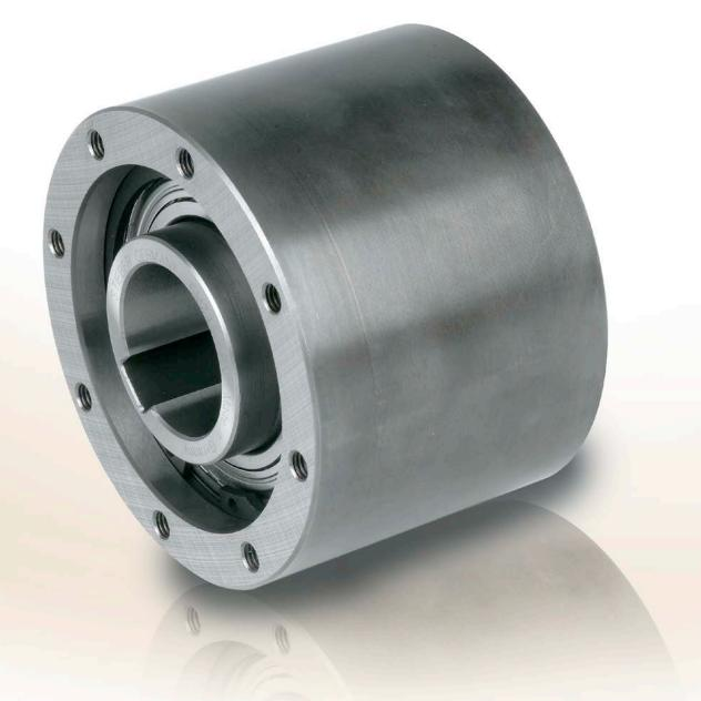
ype SMZ is a sealed, sprag type freewheel, bearing supported using two 60..ZZ series grease lubricated bearings.
